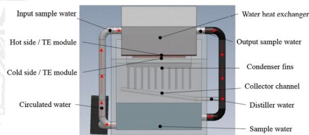
Fig. 8 : Cross-sectional view of thermoelectric distillation system and water recirculation route
