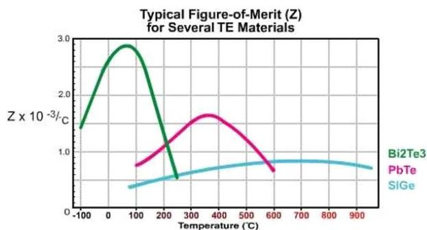
Fig. 4 : Figure of merit v/s temperature for typical thermoelectric structures
