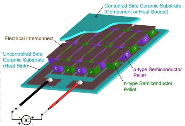
Fig. 3: Fabrication of Peltier module (Thakkar, 2016)
