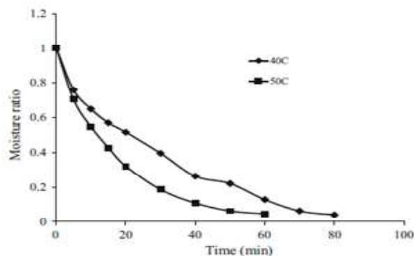
Fig. 6 : Moisture ratios of laurel clock vine leaves for selected drying air temperatures
