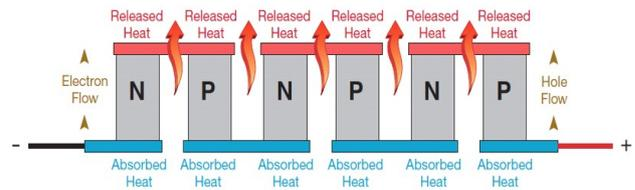
Fig. 2: Peltier cooling by multiple pellets (Thakkar, 2016)
