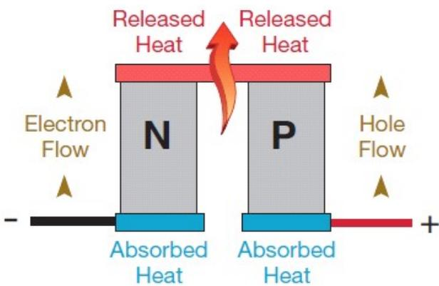
Fig.1: Peltier cooling by couple of n and p (Thakkar, 2016)
