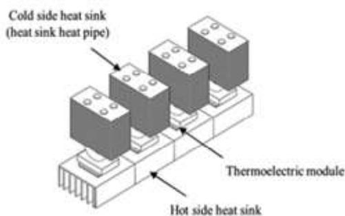
Fig. 7: Schematic diagram of the TE drying system and TE modules arrangement with rectangular fin heat sinks and heat-pipe heat sink
