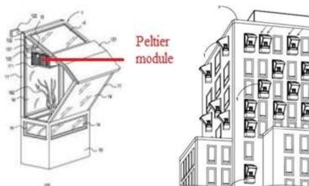
Fig. 5 : Drawings and major component of smart-green vertical greening.
