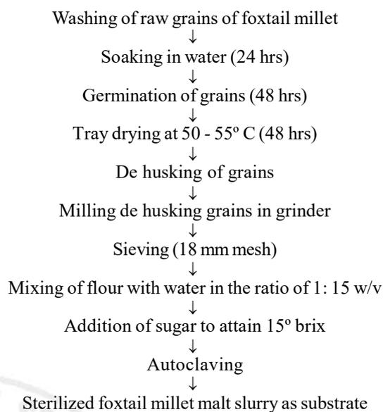
Fig. 1: Flow chart for the preparation of foxtail millet malt slurry
