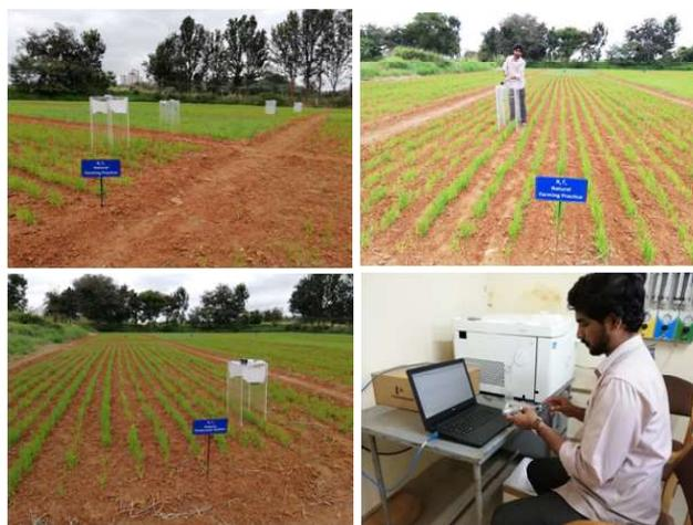
Plate 1: Collection of methane and nitrous oxide gases placed in the research plots using closed chamber technique and estimation of gases by using GCMS instrument
