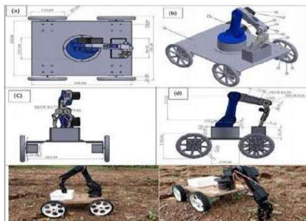
Fig. 3 : Three-dimensional CAD model of the different components of Smart seed sowing robot and actual 3D printed robot (a) Top view of the smart robot, b) Isometric view of the smart robot, (c) Front view of the smart robot, (d) Side view of the smart robot, (e) and (f) Testing of the fabricated robot in the field
