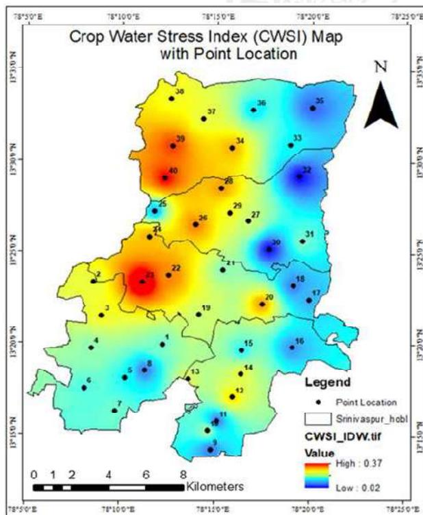
Fig. 4 : CWSI map of Srinivaspur taluk showing lowest (dark blue) and highest (red) CWSI values along with point locations where  $T_c$  measurements were made (ground truth)
