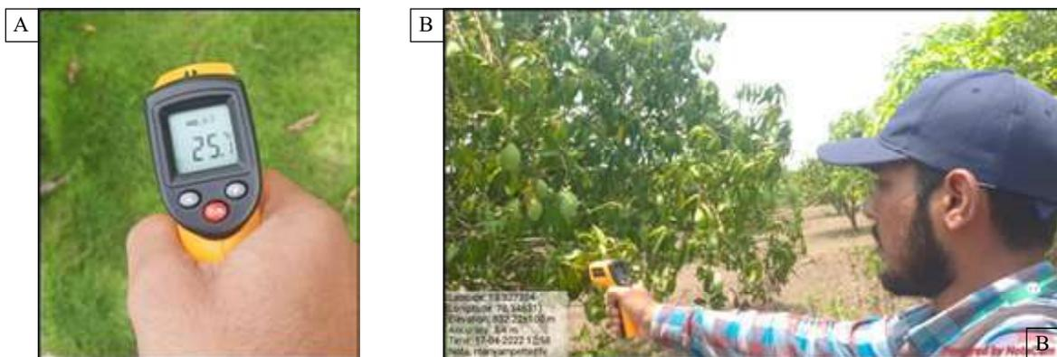
Fig. 2 : Hand-held Infrared thermometer (A) and Ground truth image (B)
