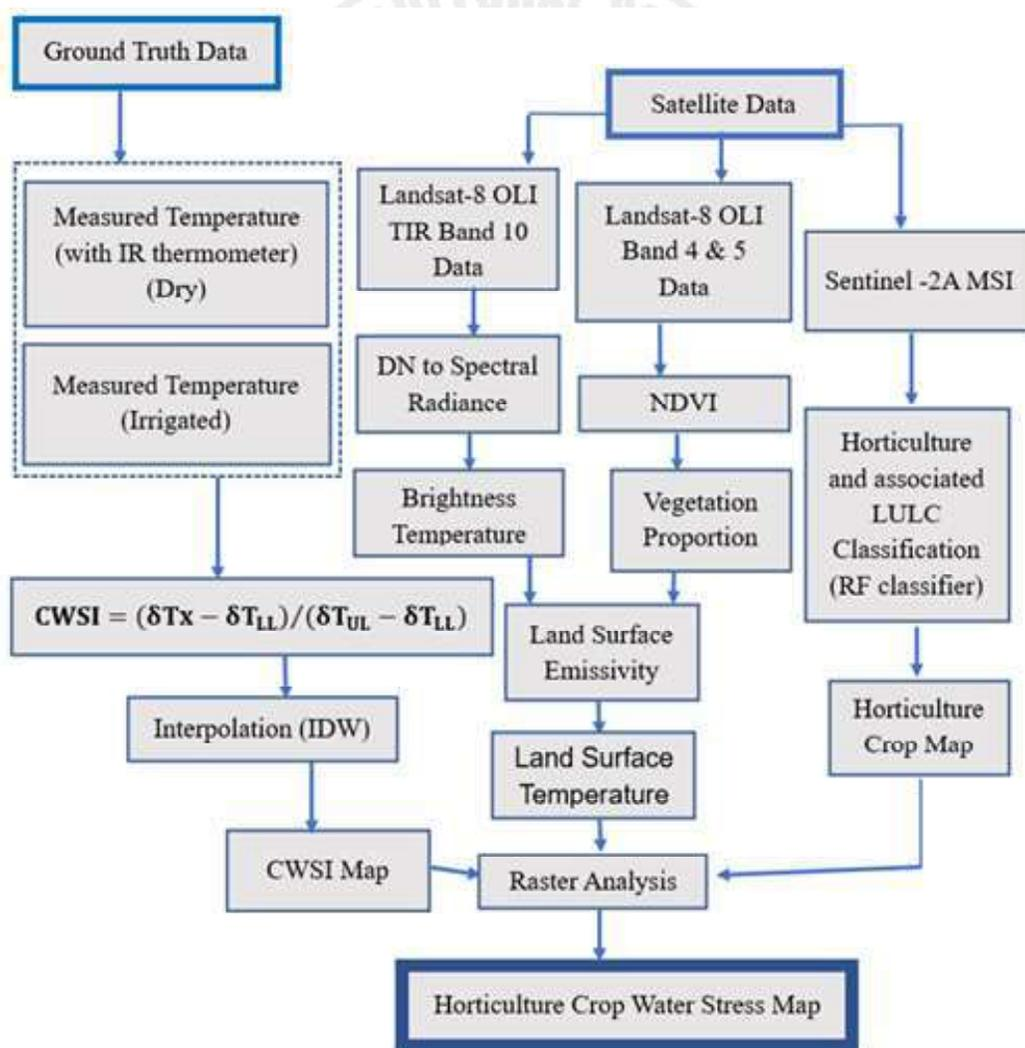
Fig. 3 : A schematic of steps involved in identification and mapping of horticulture crops affected by water stress
