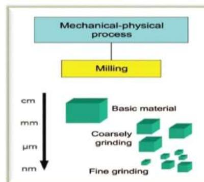
Fig. 2 : Schematic diagram for preparing nanoparticles by mechanical process
