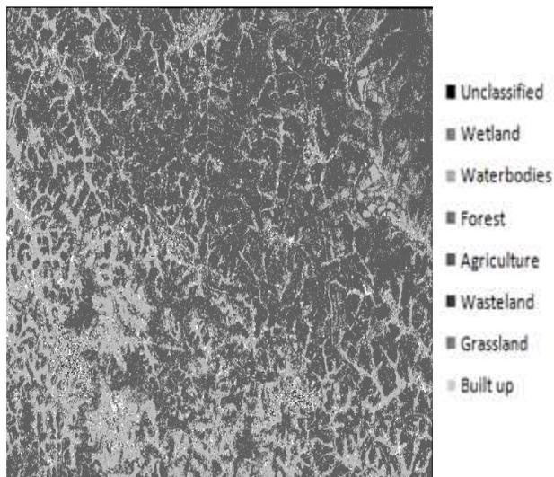
Fig. 7 : Fuzzy Classified LANDSAT - 8 Panchromatic Image with TS = 500 and VS = 167
