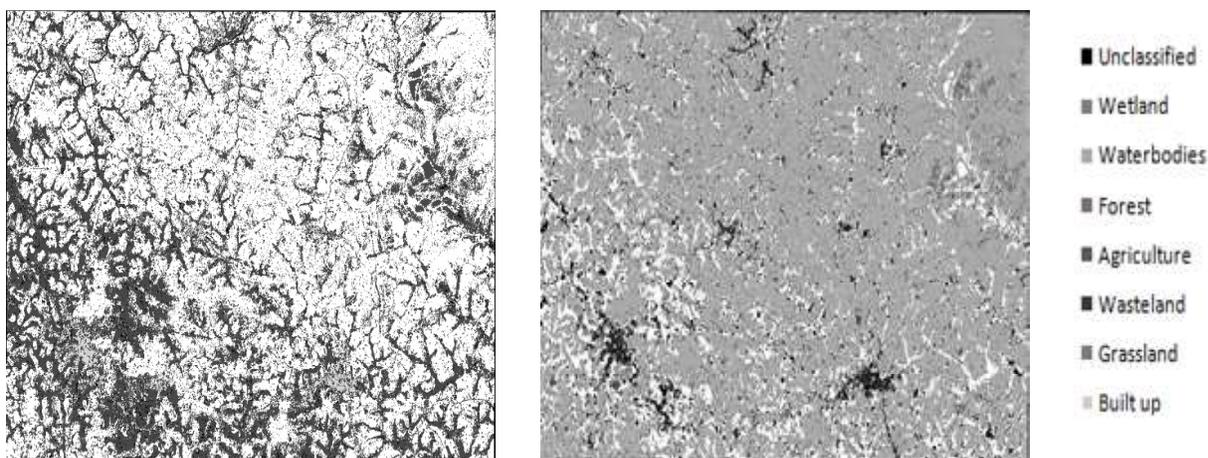
Fig. 6 : Fuzzy Classified LANDSAT-8 Panchromatic Image with TS=300, 400 and VS = 100, 136
